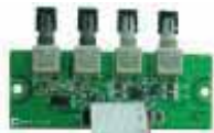
FOM-2000-SP Fiber Optics Module Mounts over the FNC-2000 Fire Network Controller Module
